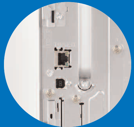
Standard USB 2.0 and 10/100BaseTX Ethernet ports make connecting to your computer quick and easy. Also available are Gigabit Ethernet and wireless options.
